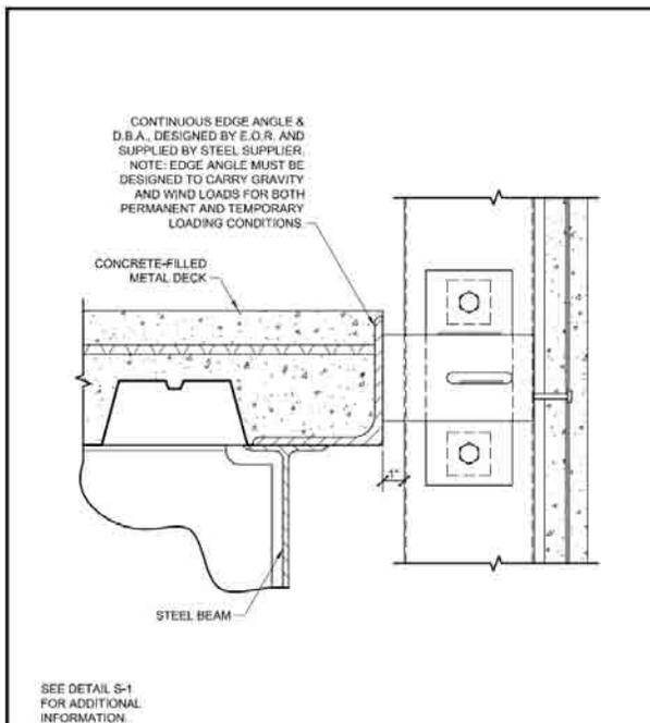
Figure D-7: Gravity Connection at Steel Edge Angle
