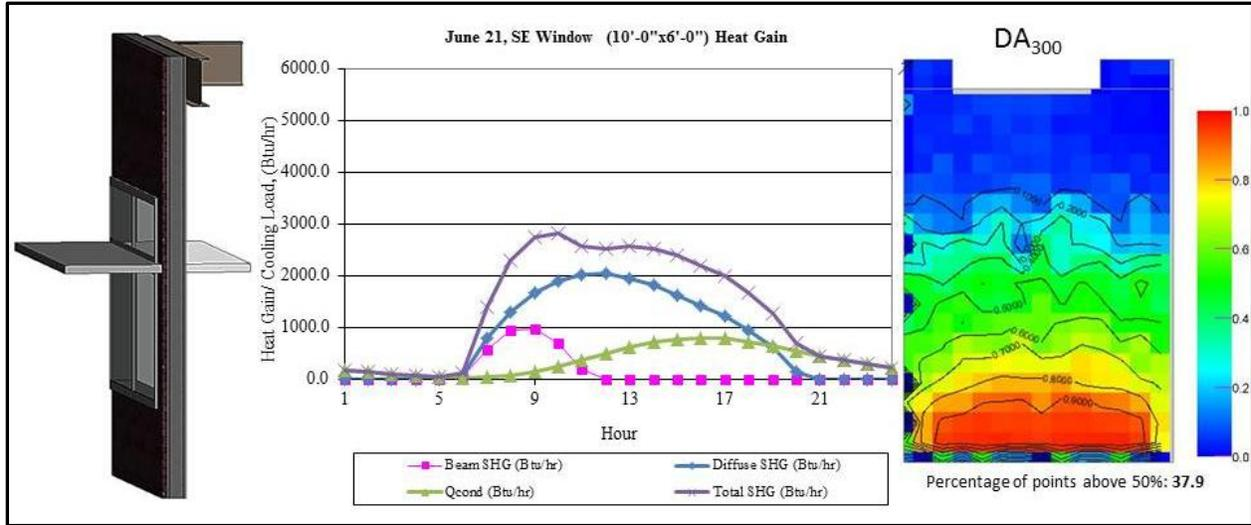
Figure D-3: Southeast-Facing Window Performance (Interior and Exterior Light Shelves)
