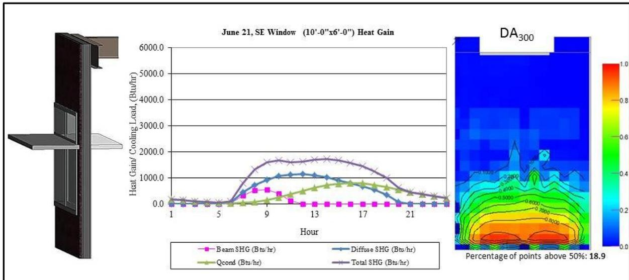
Figure D-4: Southeast-Facing Window Performance (Interior and Exterior Light Shelves with Interior Shades)
