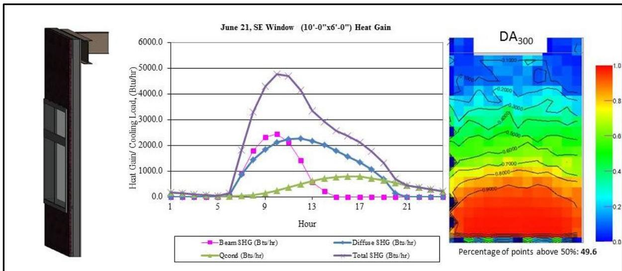
Figure D-1: Southeast-Facing Window Performance (No Window Treatment)
