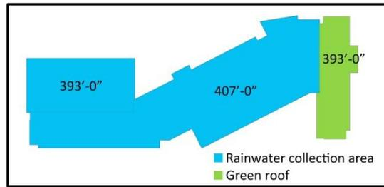
Figure 15: Roof Rainwater Collection Area
