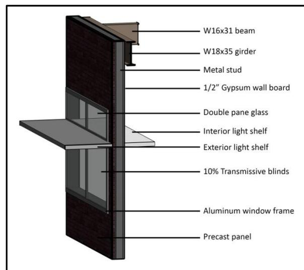
Figure 3: Integrated Façade Section from Revit
