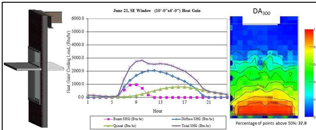
**Figure 4: Southeast-Facing Exterior and Interior Light Shelf Window Performance**
