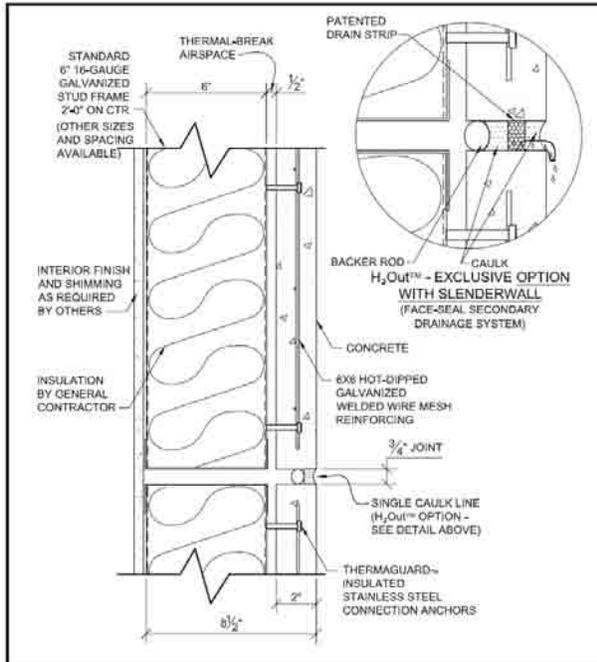
Figure D-5: Typical SlenderWall Section
