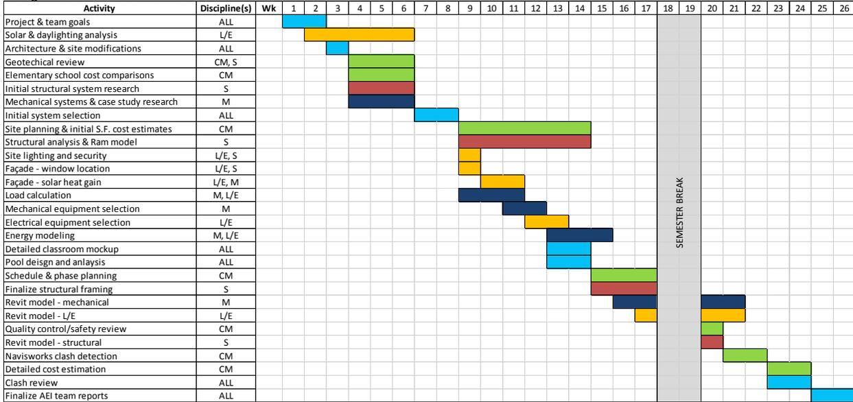
Figure B-4: Design Process Critical Path Schedule
