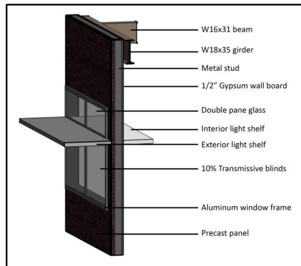
Figure 3: Integrated Façade Section from Revit
