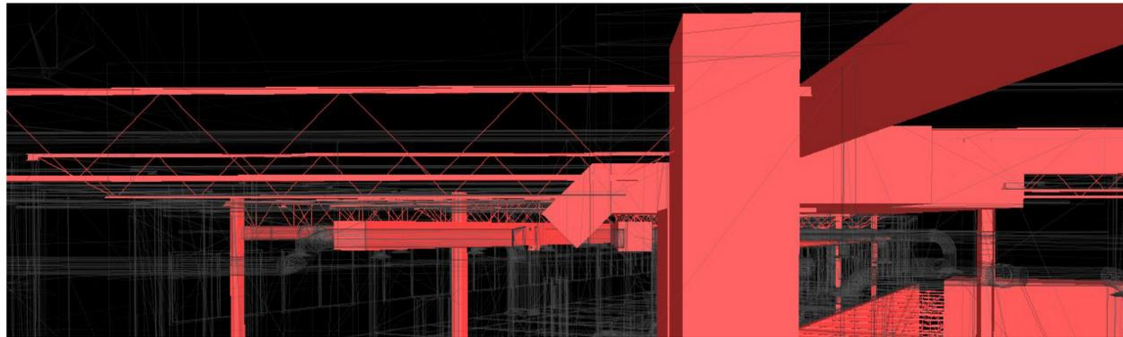
Structural/Mechanical Clash - Joist and Duct Riser
