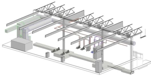
The mechanical room houses equipment that serves the building and utility connections. Specifically, it contains pumps, heat exchangers, boilers, and pool air-handling unit. The heat exchanger located within the mechanical room is connected with the geothermal loop and helps to conserve energy.
