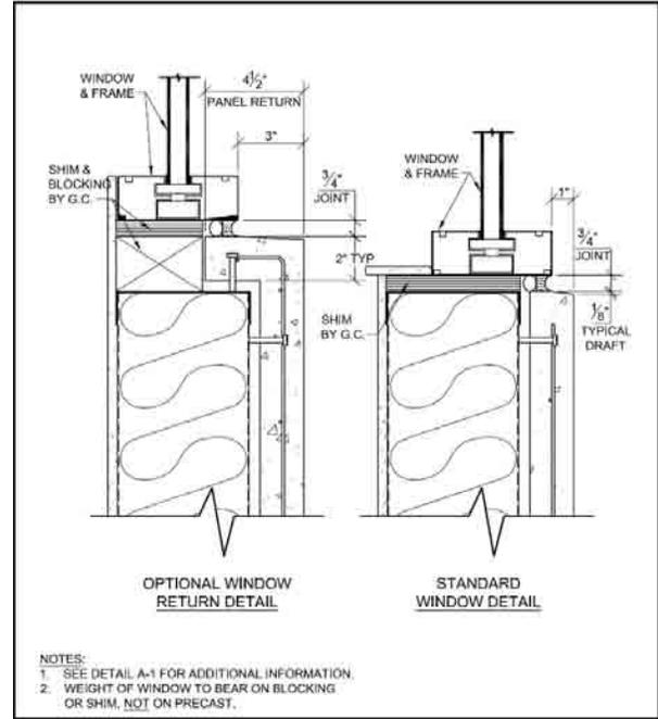
Figure D-6: Typical Window Detail
